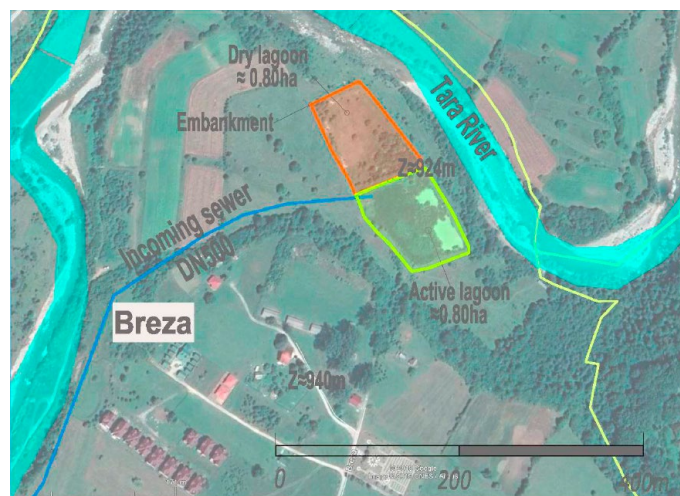
Slika 2.16. Lagune (izvor: Kolašin Wastewater Collection and Treatment - Feasibility Study Update)
